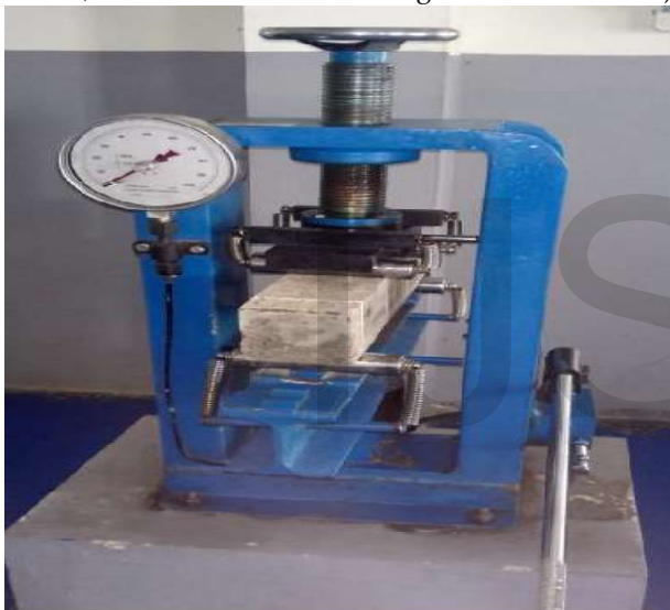
Fig.3 Flexural Strength test on beams
